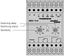
The 1-channel level control MS91-12-R monitors and regulates conductive liquid levels (II). As a dual level regulator, it can be used to control pumps and solenoid valves (I). As monitoring device it is designed for run-dry or over flow protection.
